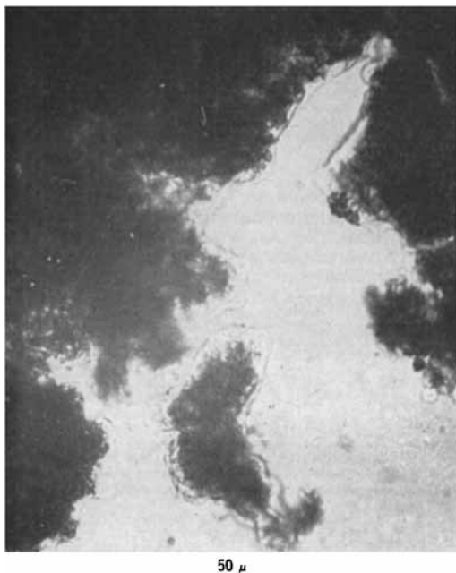
Fig. 2—Photograph of large groups of microcapsules to which 0.019% of dispersant had been added to the system.
